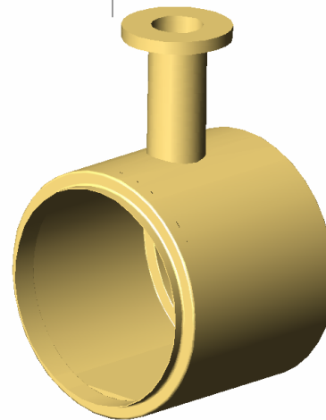
Inner support tube to isolate LH2 from Cryo-pumping ( see Option 3.1 of RAL safety requirement )
