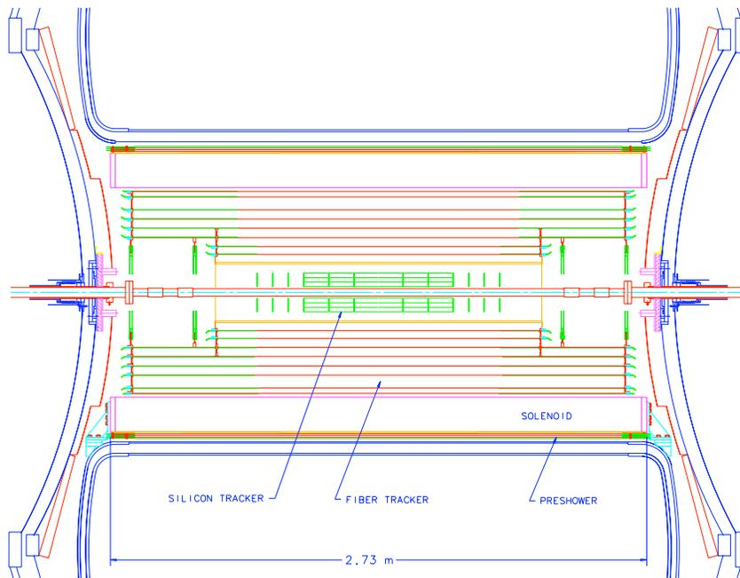
Figure 9: The DØ solenoid and central tracking system, drawn to the same scale as Fig. 8, shown as currently installed within the DØ calorimeters (from [84]).
